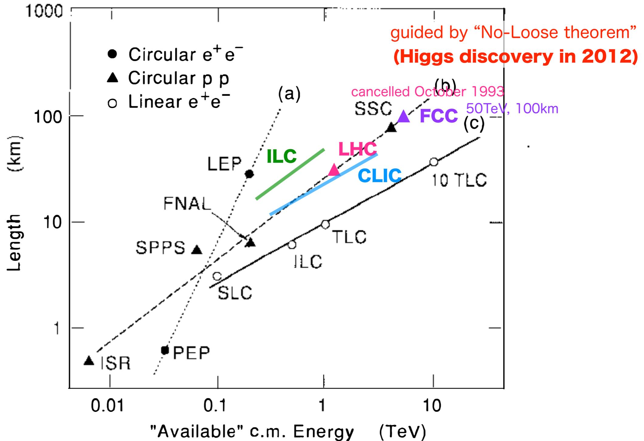
Figure 2 The "available" center-of-mass energy of various colliders, plotted against the circumference or total length of each machine. The available energy for proton or antiproton machines is taken to be one tenth of the total energy. For (a) circular electron-positron machines; (b) circular proton or antiproton machines; and (c) linear electron-positron machines.
